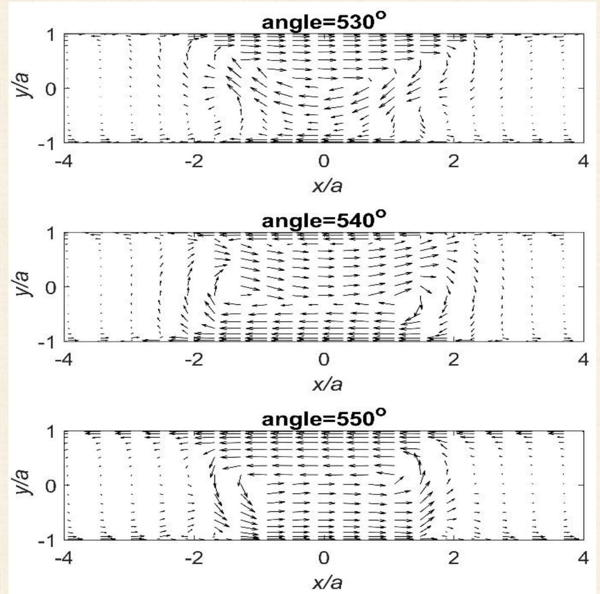
Computed sheet current density for three rotor positions,  $h_0 / j_c^0 = 10$
