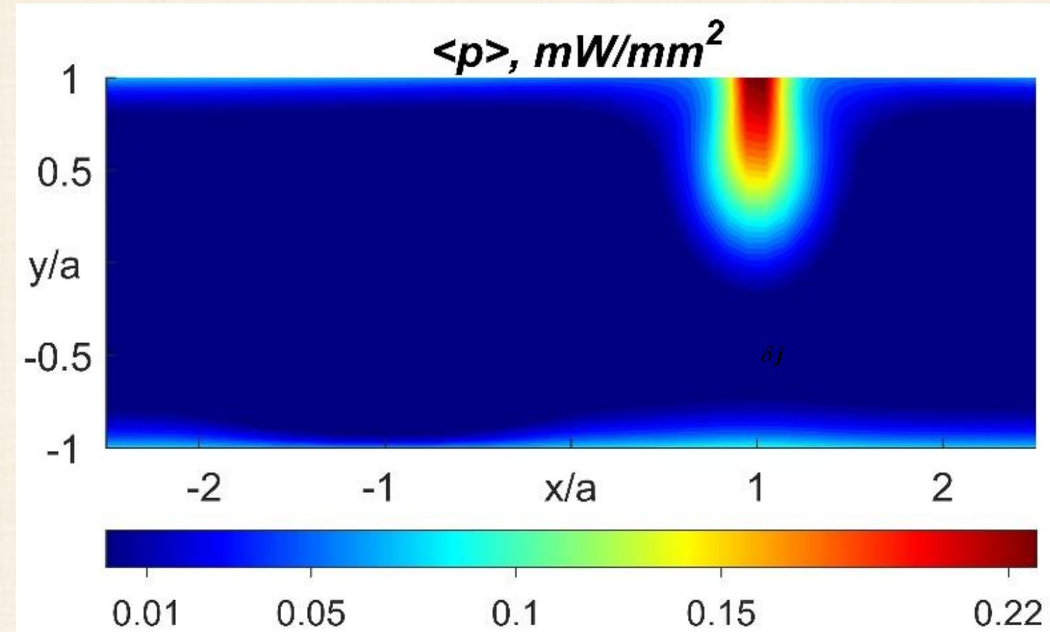
The time-averaged loss power density  $\langle p \rangle$ , high in the lower sheet critical current density area.
