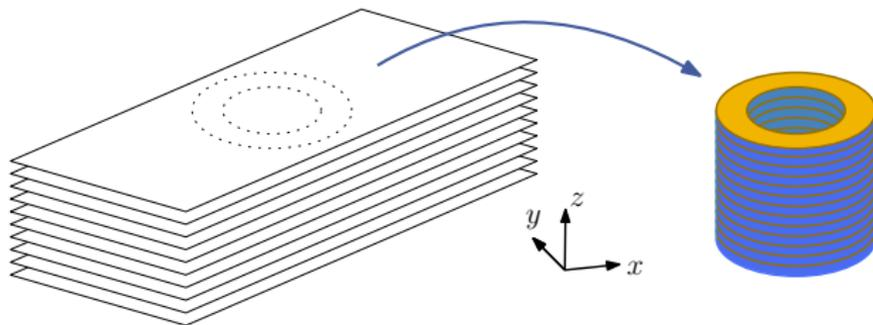
Inner radius: 13 mm. Outer radius: 22.5 mm. Height: 14.9 mm.
