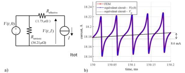
Fig. 2. a) complete time-domain empirical equivalent circuit of the flux pump taking internal dissipation into account, b) Detail of the current during 5 cycles.
