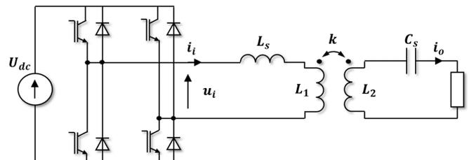
Fig. 1. Lumped circuit model of HTS wireless power transmission system.
