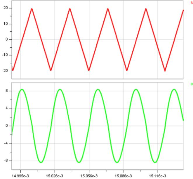
Fig. 2. Current waveforms obtained from lumped circuit model. Current of transmitter (red), and receiver (green).
