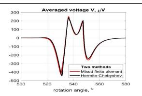
Fig. 2 The voltage induced during the second rotor rotation computed by the mixed finite element method [6] and using the spectral Hermite-Chebyshev method.
