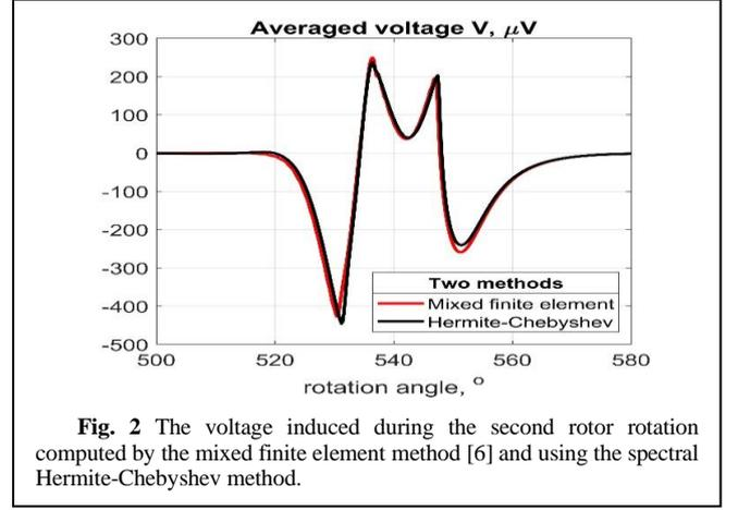
**Fig. 2** The voltage induced during the second rotor rotation computed by the mixed finite element method [6] and using the spectral Hermite-Chebyshev method.
