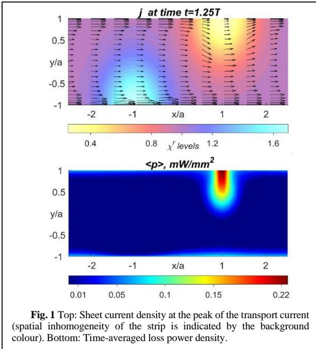
**Fig. 1** Top: Sheet current density at the peak of the transport current (spatial inhomogeneity of the strip is indicated by the background colour). Bottom: Time-averaged loss power density.
