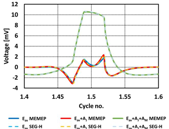
Fig. 3. Comparison of the three voltage components of the output voltage:  $l \cdot E_{av}$  and the two contributions to the vector potential  $A$  from the current density in the HTS wire,  $A_J$ , and permanent magnet,  $A_M$  [17].
