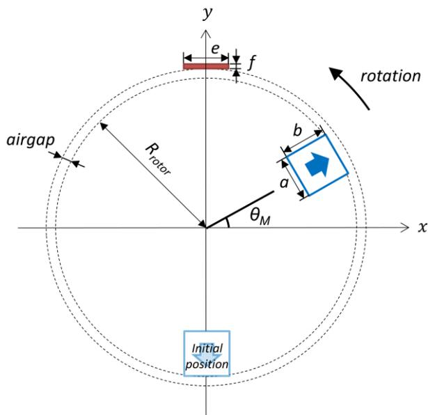
Fig. 2. Geometry of the HTS dynamo benchmark problem [8]. A permanent magnet rotates anticlockwise past a (stationary) HTS wire.
