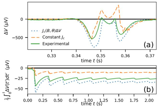
Fig. 1. (a) Open-circuit voltage waveforms for the HTS dynamo presented in [6] for the  $\mathbf{H}$ -formulation + shell current model using measured in-field  $J_c(B, \theta)$  data for the HTS wire or a constant  $J_c$  assumption, compared with experimental results. (b) Cumulative time-average for each waveform, which converges to  $V_{DC}$  in each case at  $t \rightarrow \infty$ .
